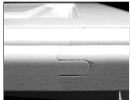
Example of door end joint separation
